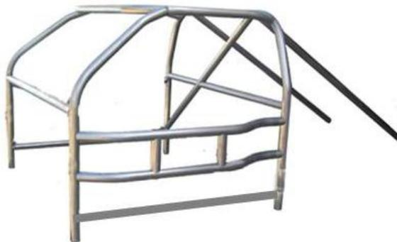
8. Roll-cage Steel Tubing and Hardware (Vehicle Weight Without Driver):
