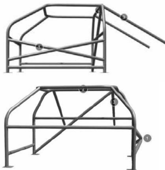
Basic “X-Bar” Style Door Bar Roll Cage
