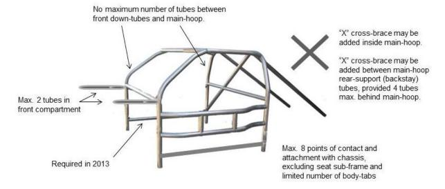
Teams MAY exceed the design and application of the "maximum, value-free" roll-cage; however, additional value will be assessed by the Tech Inspector, based on the perceived performance enhancement of the roll-cage. As per Section 3.2 of ChumpCar's Basic Competition Rules:
