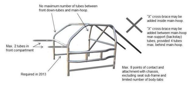
Teams MAY exceed the design and application of the "maximum, value-free" rollcage; however, additional value will be assessed by the Tech Inspector, based on the perceived performance enhancement of the roll-cage. As per Section 3.2 of **ChumpCar's Basic Competition Rules:**
